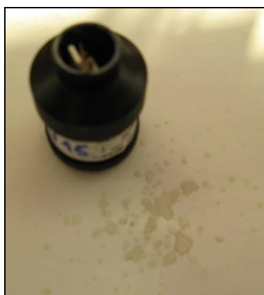
Fig 18.18-3: Drops of electrolyte from the N15 sensor after -30 and +70 storage and drop tests
