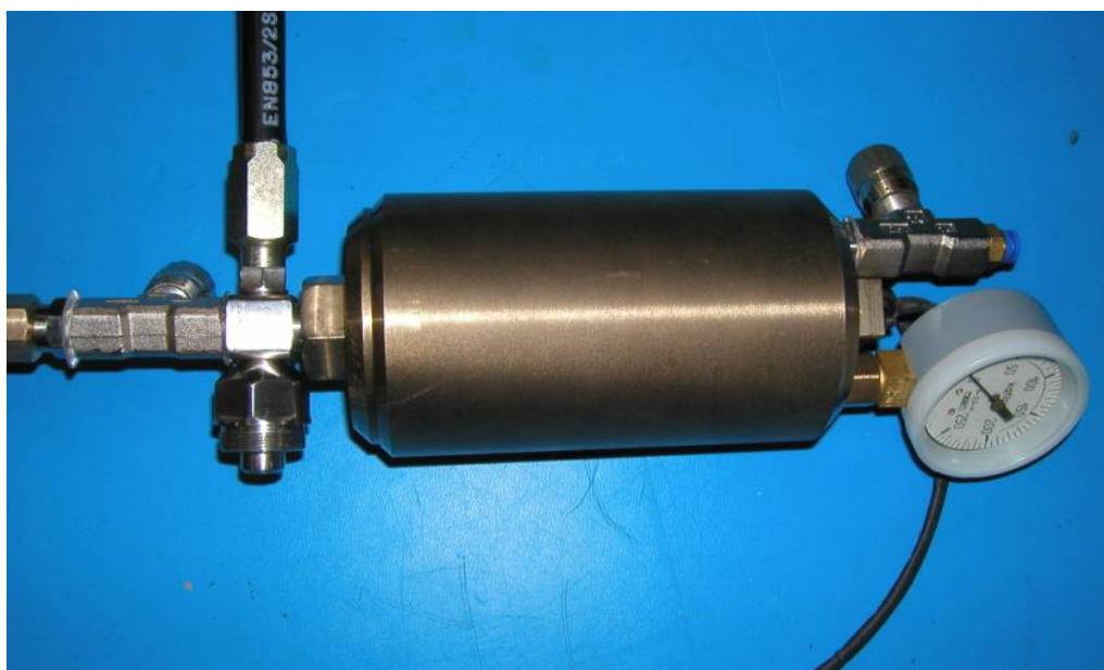
Fig 18.11-1. Chamber for Test 9. The gauge is for safety purposes only: all readings are taken via the digital sensors.
