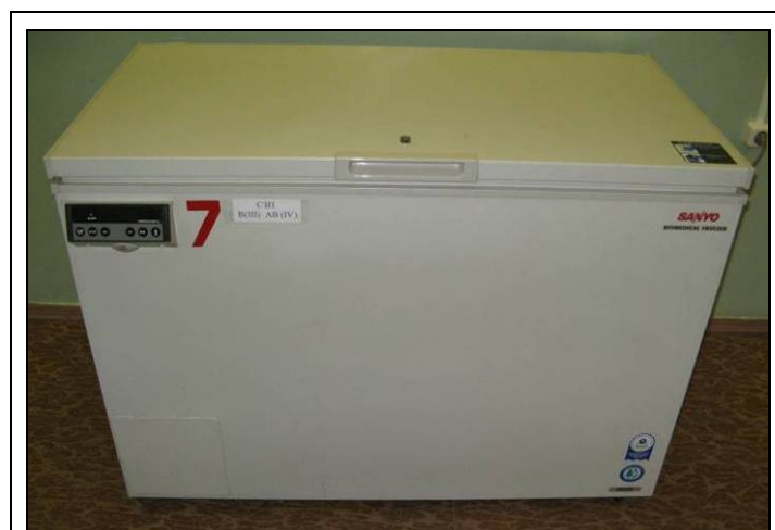
Fig 18.16-1. Biomedical freezer for testing of the equipment. The freezer power is 220W. Effective capacity is 426 litres.
