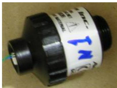
Fig 19.1-1. Sensor marking. Sensor 1 had an output mean of 11.94 mV in air at a mean temperature of 24.91 C. All others were in the range 11.85 to 12.0mV under similar conditions.
