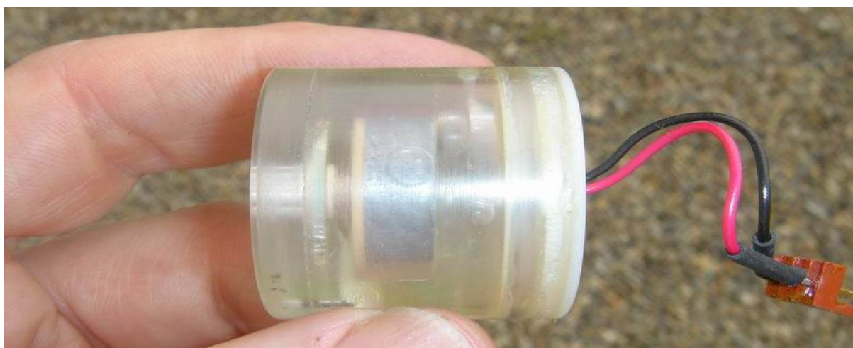
Fig 15.1-3: Insovt DK-32 showing KOH solution fill: bubble can be seen behind anode and also in second compartment. This shows the two part potting process to avoid contaminants affecting the cell. Note the thick material in front of the cell to prevent depressurisation forcing electrolyte out.
