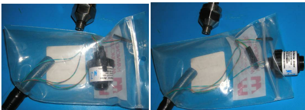
Fig 18.12-1. PPO2 sensor in/out of plastic chamber with CO2 feed.
