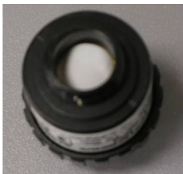
Fig 18.8-2. Broken PPO2 sensor. Part of the membrane is out of the housing.
