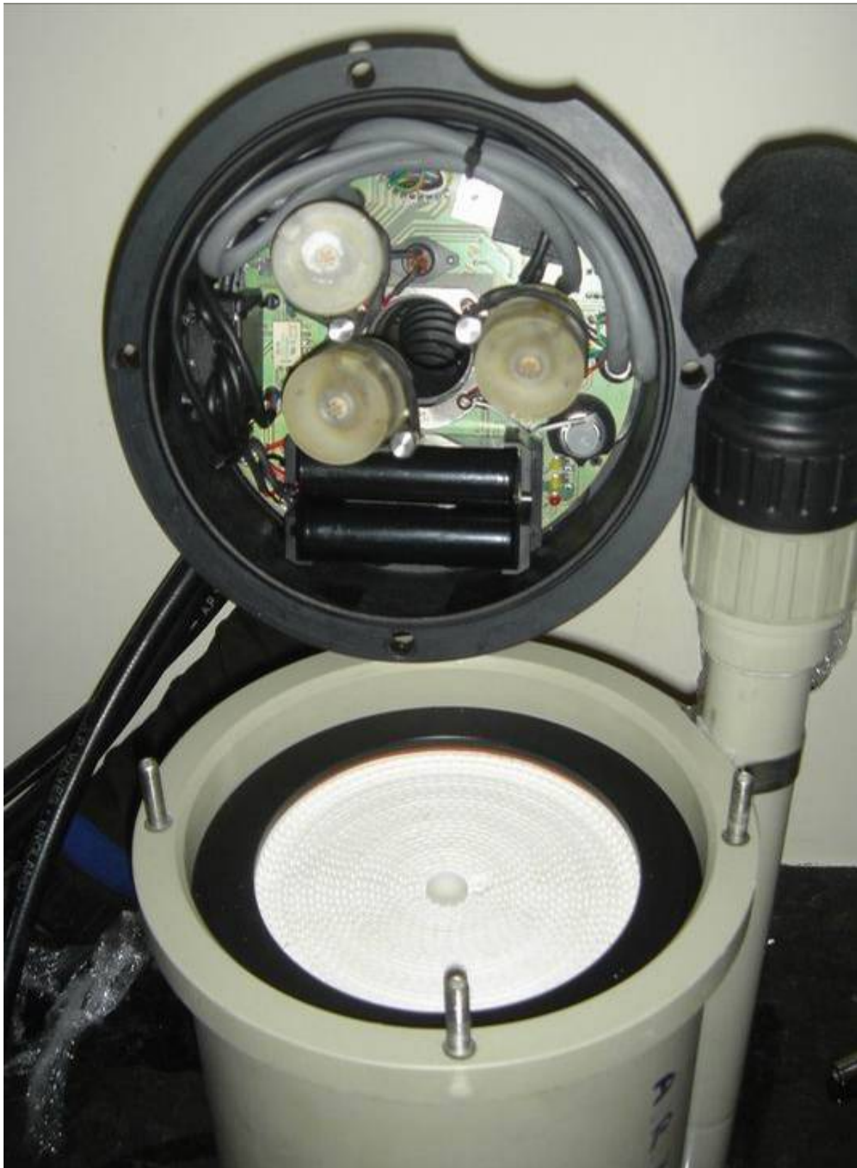
Fig 15.1-5: Test Rig using an improved AP Valves Inspiration Classic to test the Insovt DK.32s on dives. An ExtendAir scrubber was fitted, the batteries were replaced by rechargeable lithium ion cells and the failure point at the top of the lid was removed by Deep Life.
