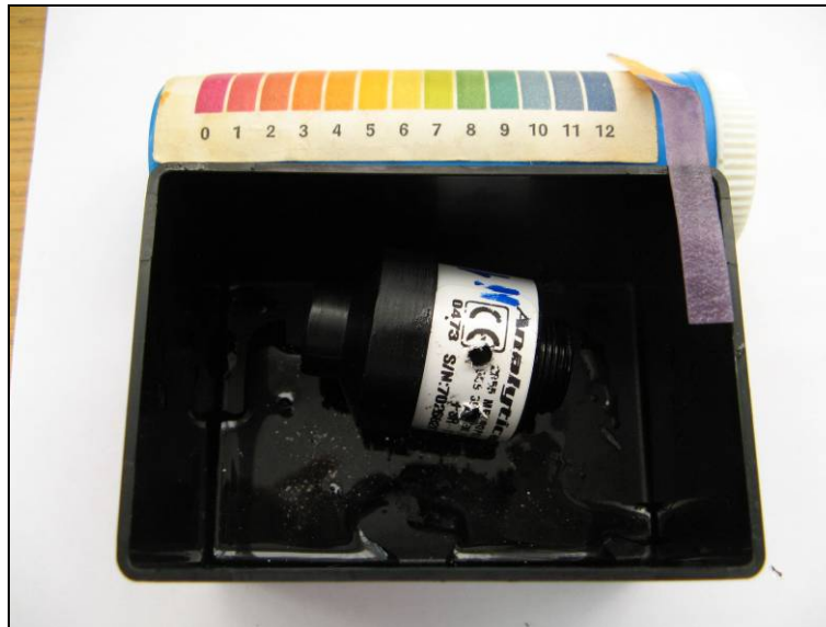
Fig 18.20-1: Sensor losing electrolyte.
