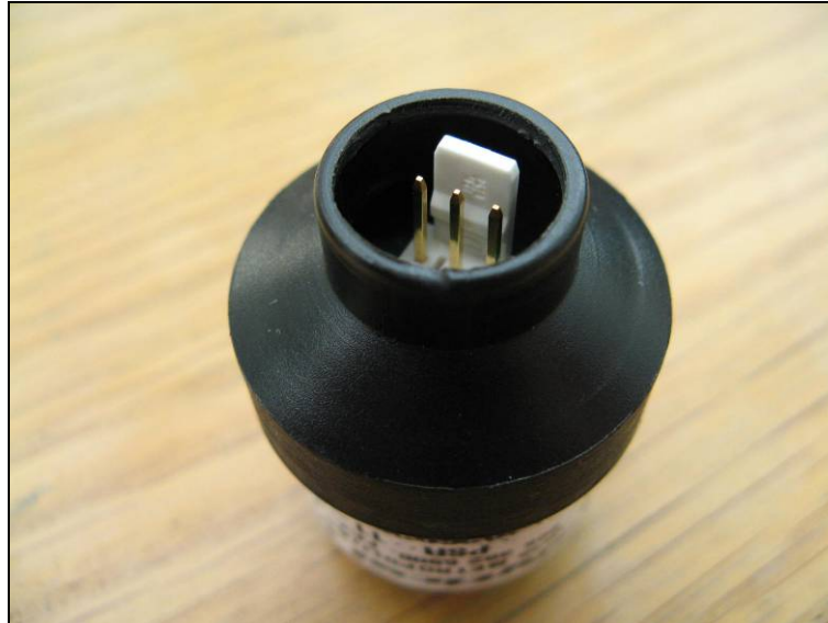
Fig 18.18-4: A small dent can be seen is near the connector hole of the N14 sensor
