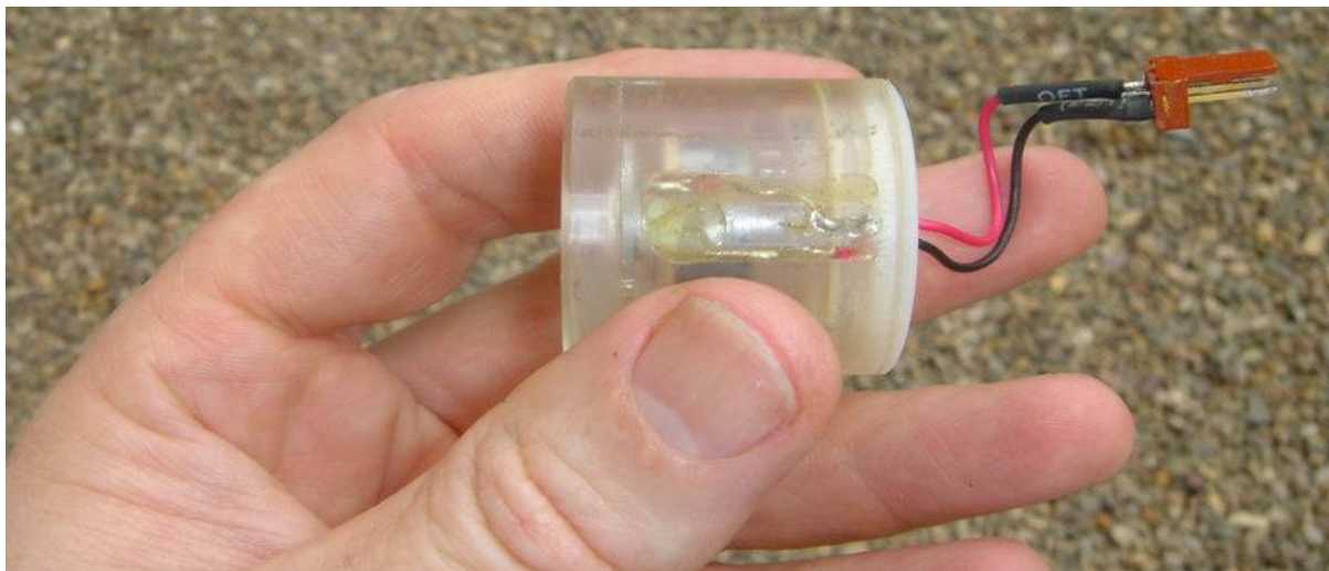
Fig 15.1-2: Side view of Insovt DK-32 after testing, showing the hard wired temperature compensation circuit potted into housing.
